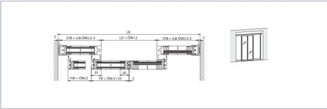
Installation: Cantilevered installation
