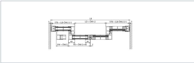
Installation: Cantilevered installation
