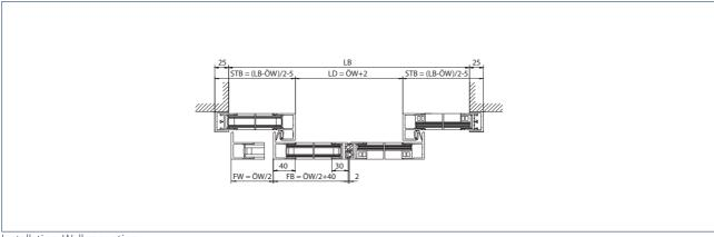
Installation: Wall mounting LB = Clear overall width STB = Width of side parts LD = Clear passage FW = Travel path
