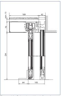
Floor guide: Pointwise with reinforced supporting bracket
