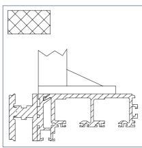
Carrier and running rail additionally suspended from the ceiling
