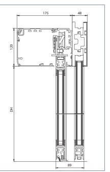
High cantilevered carrier DH = Passage height
