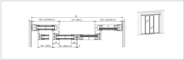
Installation: Cantilevered installation
