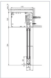
Floor guide: For floor mounting DH = Passage height
