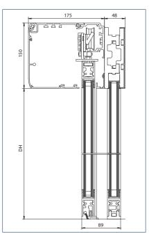
Low cantilevered carrier DH = Passage height
