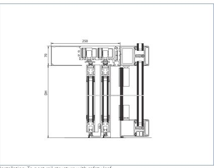
Installation: To post-rail structure with safety leaf
