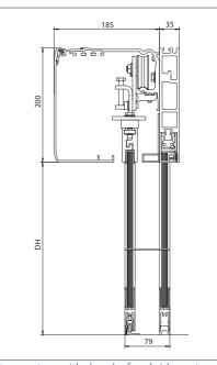
Door system with door leaf and side parts under carrier
