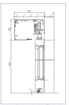
Version with 120 mm hood and floor guide for floor mounting
