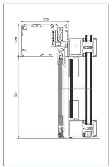
Installation: To post-rail structure with safety leaf
