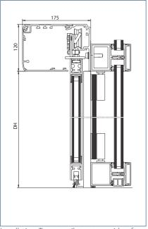
Installation: To post-rail structure with safety leaf
