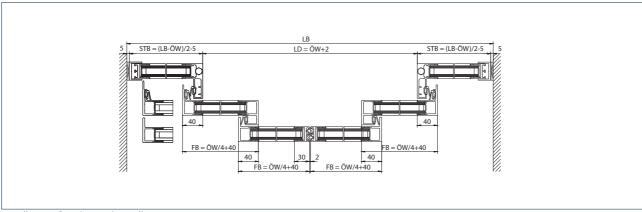
Installation: Cantilevered installation
