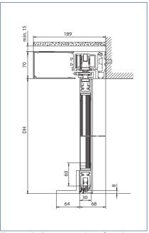
Floor guide: Pointwise with reinforced supporting bracket
