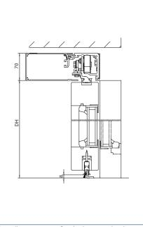
Installation variant for thicker wooden leaves and floor guide for floor mounting
