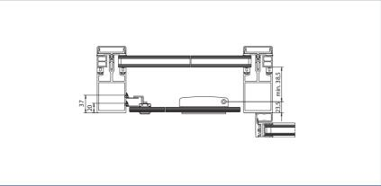
Installation: To post-rail structure with safety leaf
