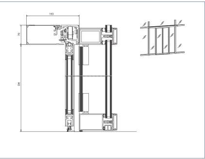
Installation: To post-rail structure with safety leaf
