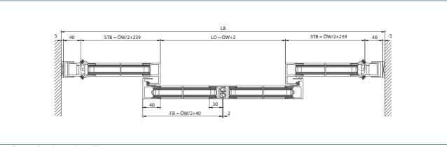
Installation: Cantilevered installation
