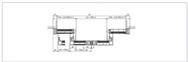
Installation: Wall mounting with side parts
