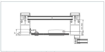
Installation: To post-rail structure with safety leaf
