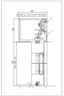
Version with 150 mm hood and floor guide for floor mounting
